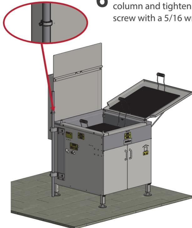
**7** Slide the straight-arm section onto the column.
