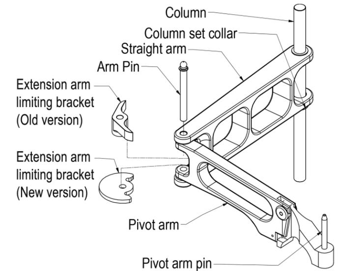
**6** Slide the set collar onto the column and tighten the set screw with a 5/16 wrench.
