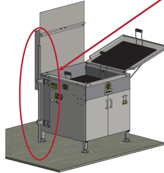
**3** Align the holes in the column mounting brackets, with the holes in the fryer frame assembly.
