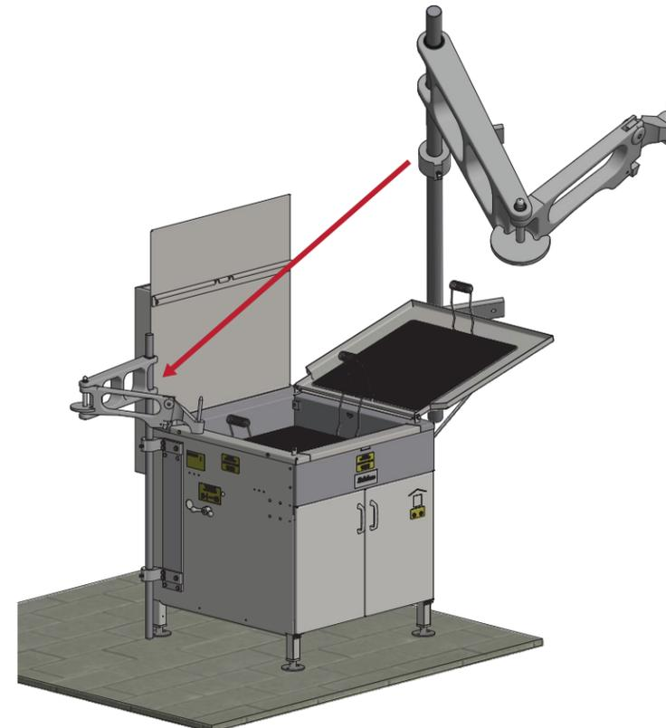
**8** Put the pivot arm section between the legs of the straight arm.
